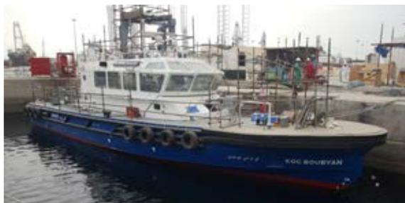
**G**randweld Shipyard in Dubai is nearing completion of their 6-boat build programme of Camarc 23m Pilot boats for Kuwait Oil Company. The 23m steel series feature the Camarc refined hull form for improved efficiency and comfort. During trials speeds of 24 Knots were achieved, exceeding the contract requirements. The wheelhouse layout has been optimised and configured for a 3 crew + 15 passenger capacity.
