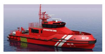
Two Camarc 25m Fire Boats for the Hellenic Fire Service are also building at the Tehnomont Shipyard. Powered by a triple Hamilton waterjet installation, fitted with the Hamilton JETanchor system and a bow thruster to facilitate station keeping. The main propulsion engines will be utilised to provide both station keeping and firefighting capabilities at the same time, without the need for additional engines to install & maintain.
