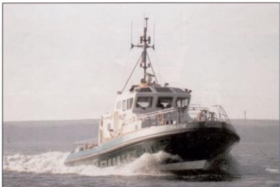
The Camarc-designed 19m 20knot steel pilot boat delivered to Milford Haven at the end of 2000.
