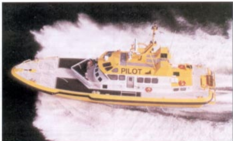
The Columbia River Bar pilot vessel Chinook , built in aluminium by Kvichak Marine, with a unique self-righting capability.
