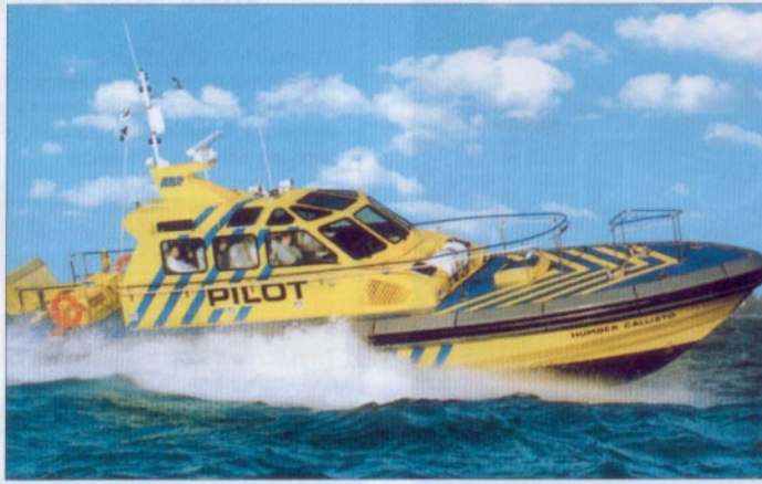
Three Scania D14 engines powering triple water jets push the 17m 'Humber Callisto' to 36 knots.
